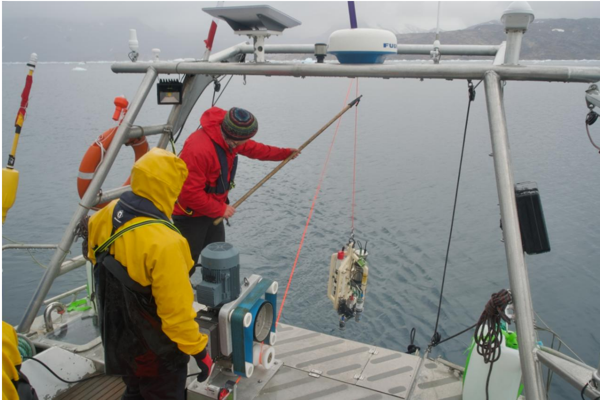
Figure 6. Profiling operations. During a typical profiling activity, one crew was responsible for controlling the winch while another assisted the winch by lifting the profiler and stabilizing it with a gaff. The profiler was retrieved at a slightly faster rate ( \sim 0.8 m/s), during which crew members shared the responsibility of spooling back the Dyneema rope. Photo: Matthieu Klitting
