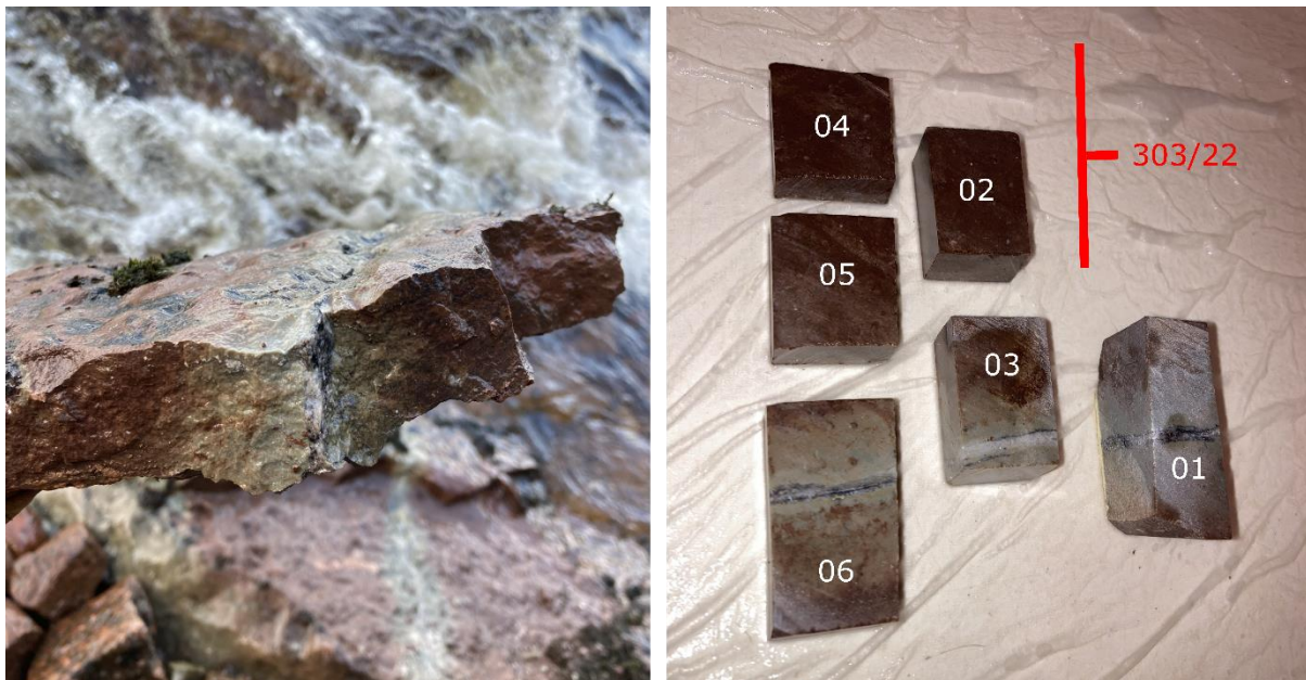
Figure 2.2. Rock sample from the study site (left), and the six pieces prepared for thin section with their orientation (right).
