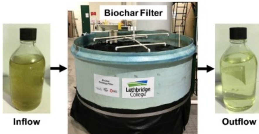
Figure 11 , (Khiari et al., 2020): Contaminated water before (inflow) and after (outflow) being processed through a biochar filter.
