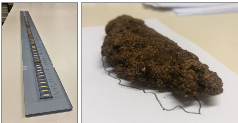
Figure 2. The images show the ashed sample boats prepared for XRF-CS analysis (left) and a dried peat sample during tracing for bulk density measurements (right).
