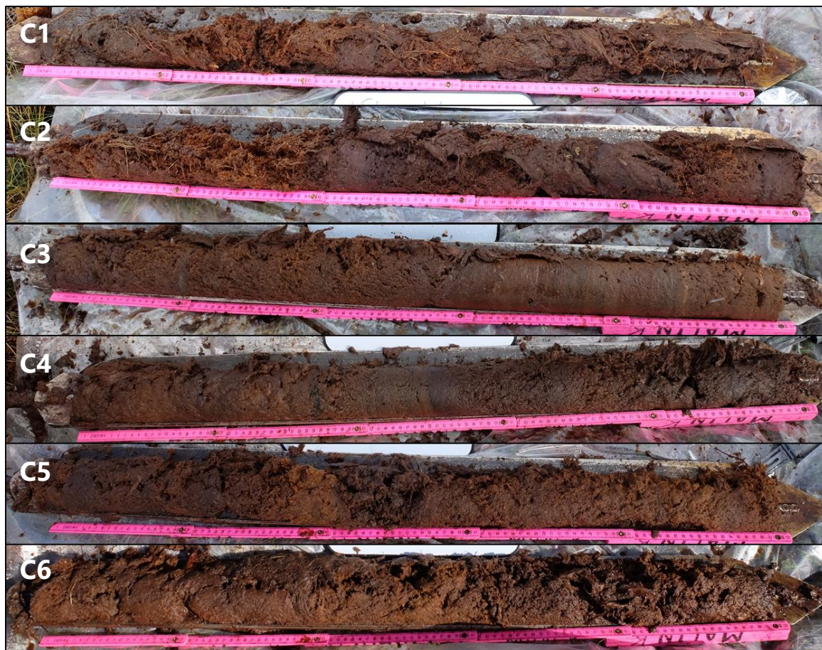
Figure 14. Images of fresh core sections of the SMDS core taken from two alternating holes. From the top the sections cover deposit depths C1) 20-120 cm, C2) 50-150 cm, C3) 125-225 cm, C4) 200-300 cm, C5) 275-375 cm and C6) 350-450 cm.
