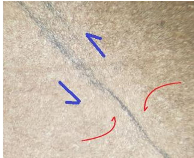
Figure 8: The figure (left) shows shearing along the black vein in x100 magnification, see red arrows for shear sense and blue for suggested direction (sinistral shear).
