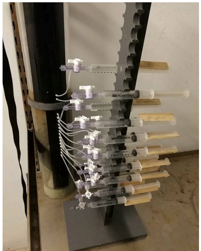
Figure 3. Picture showing pore water extraction using the rhizon method. Sticks were added to the syringes pistons to get sucked back in to the syringes.
