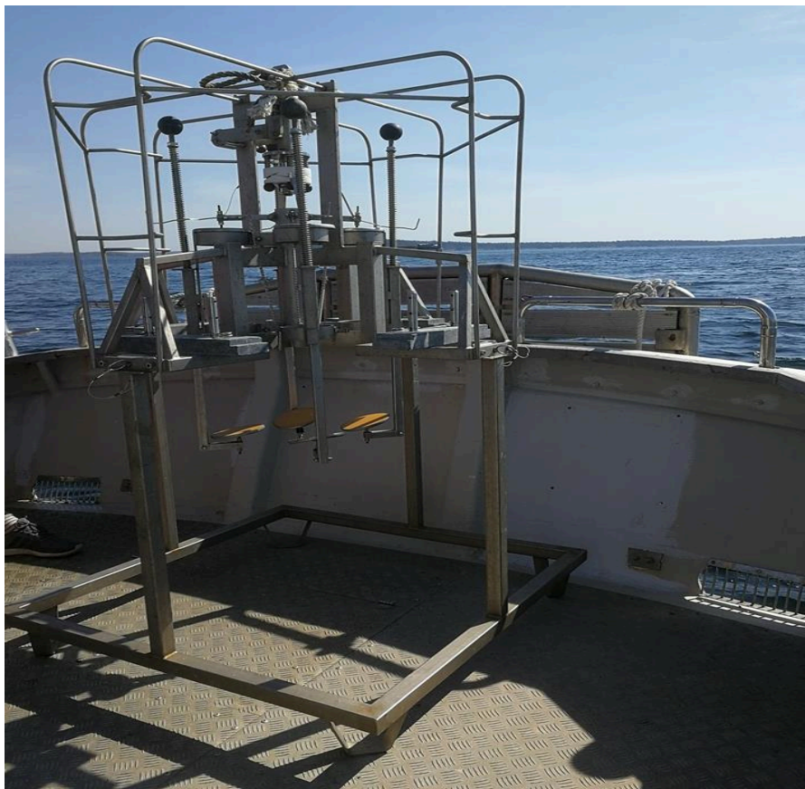
Figure 2. Picture showing multi-corer used during sampling.
