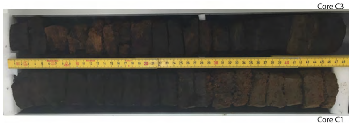
Figure 4 shows the sediment samples from SEK2016 core 1 (bottom) and SEK2016 core 2 (top) reconstructed to a continuous sequence. The top of the core is at 0 cm (left).
