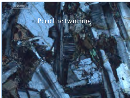
Image P2: Plagioclase and potassium feldspar. Upper left: Carlsbad twins. Upper right: albite twinning. Lower left: pericline twinning. Lower right: partially developed tartan twinning. Horizontal field of view for the upper left image is 5.6 mm. Horizontal field of view for the other three images is 1.4 mm.
