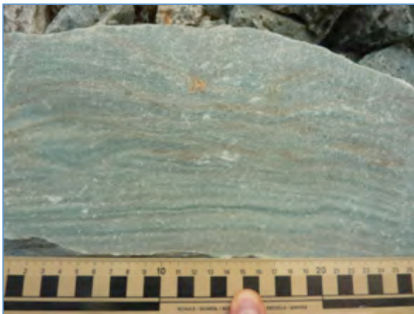
Image S10: Structures in outcrops, of possible sedimentary origin. Possibly flaser bedding or even lenticular bedding. The dark blue layers are presumably more mud-rich than the light blue layers as they are more alumina-rich. Some scour-and-fill structures are also possibly present; the most distinct one can be found below the label.
