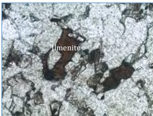
Image P7: Ilmenite and scorzalite (aluminium phosphate) in the kyanite rock. Upper row: scorzalite under cross-polarized and plain polarized light, respectively. Lower row: ilmenite under similar lightning conditions. Horizontal field of view for all images is 1.4 mm.
