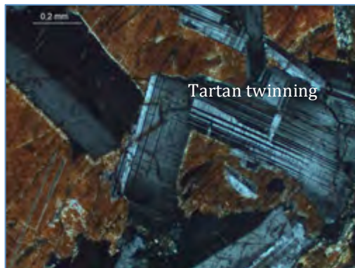
Image P2: Plagioclase and potassium feldspar. Upper left: Carlsbad twins. Upper right: albite twinning. Lower left: pericline twinning. Lower right: partially developed tartan twinning. Horizontal field of view for the upper left image is 5.6 mm. Horizontal field of view for the other three images is 1.4 mm.
