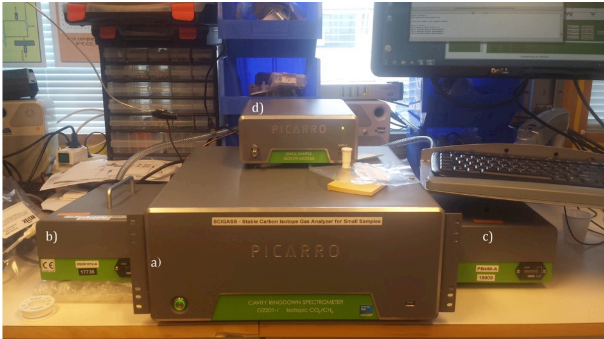
Figure 2.5 - The Picarro set up in the lab with a) the Picarro analyzer, b) external pump for the SSiM, c) external pump for the Picarro analyzer, d) the SSiM with a tedlar bag connected.
