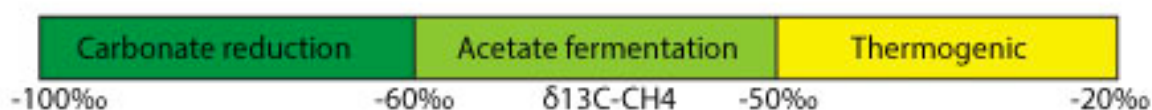
Figure 1.2 - the boundaries of the \delta^{13}\text{C} signal with respect to formation environment based on information from Whiticar 1999.
