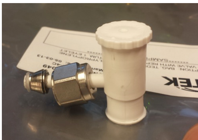
Picture 3.2 the modified tedlar bag used for injection sample into the SSiM
