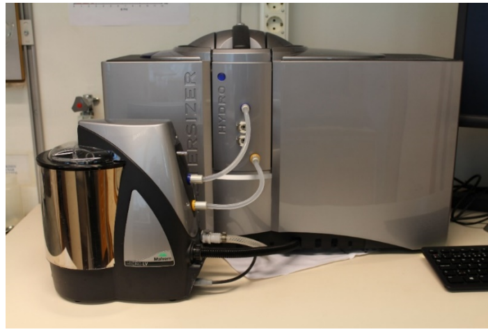
Figure 4. The above photo shows the Malvern Mastersizer 3000 which was used for the grain size analysis. Photo taken by César Fuentes Guerrero.
