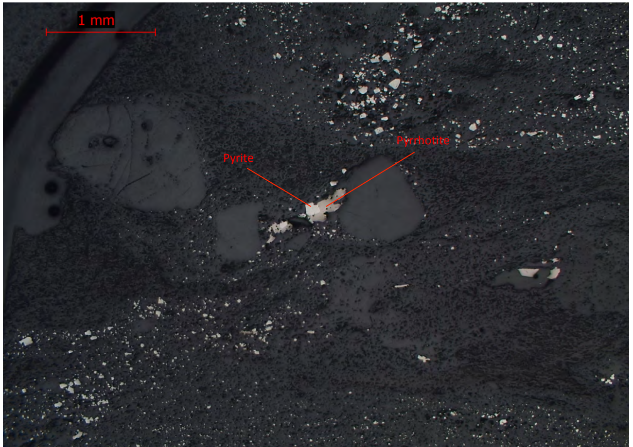
Fig.21. Small grains of pyrite and pyrrhotite in a matrix of quartz, carbonate and actinolite. Several large clasts of quartz and carbonate occur in the matrix. The marked pyrite and pyrrhotite are in the pressure shadow between two clasts because of deformation.
