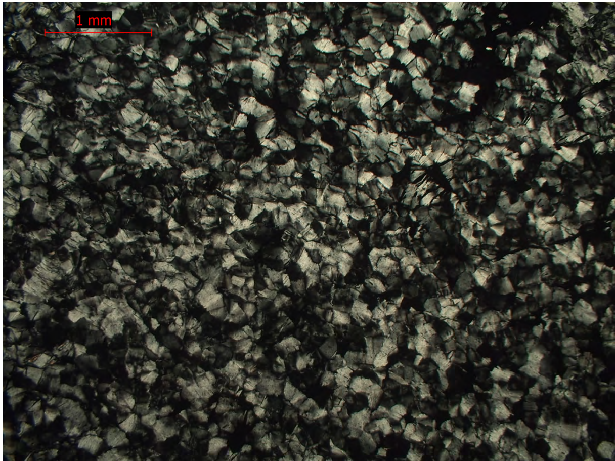
Fig.19 Chlorite with fan texture.
