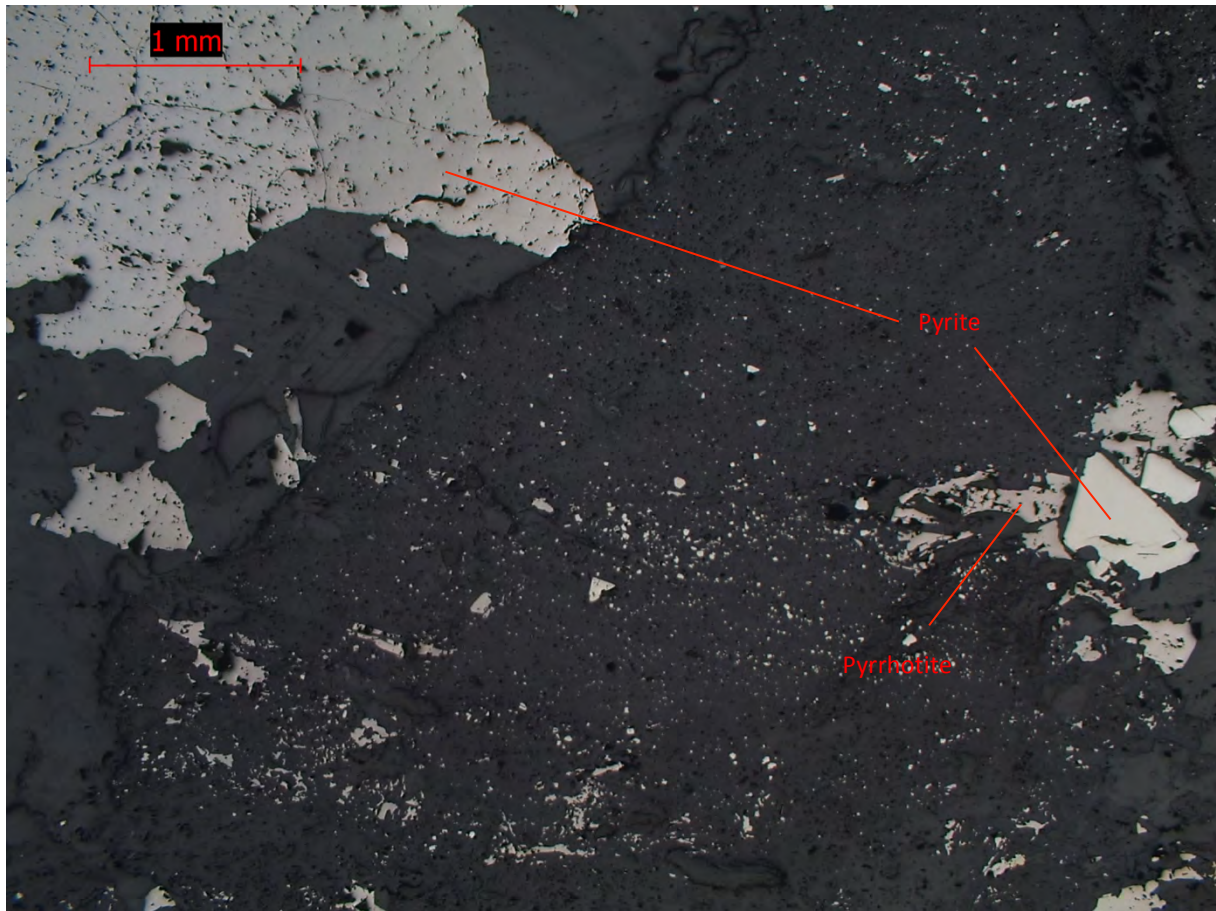
Fig.20. Grains of pyrite and pyrrhotite in different sizes in a matrix of quartz, carbonate, chlorite and biotite. A big clast surrounds the big pyrite grain.
