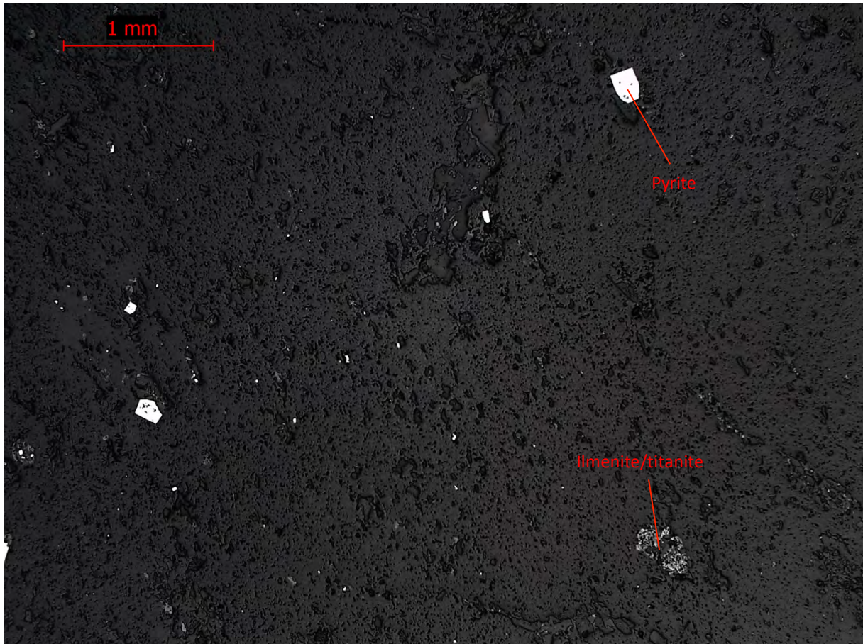
Fig.4. Pyrite and ilmenite/titanite in a matrix of host rock.
