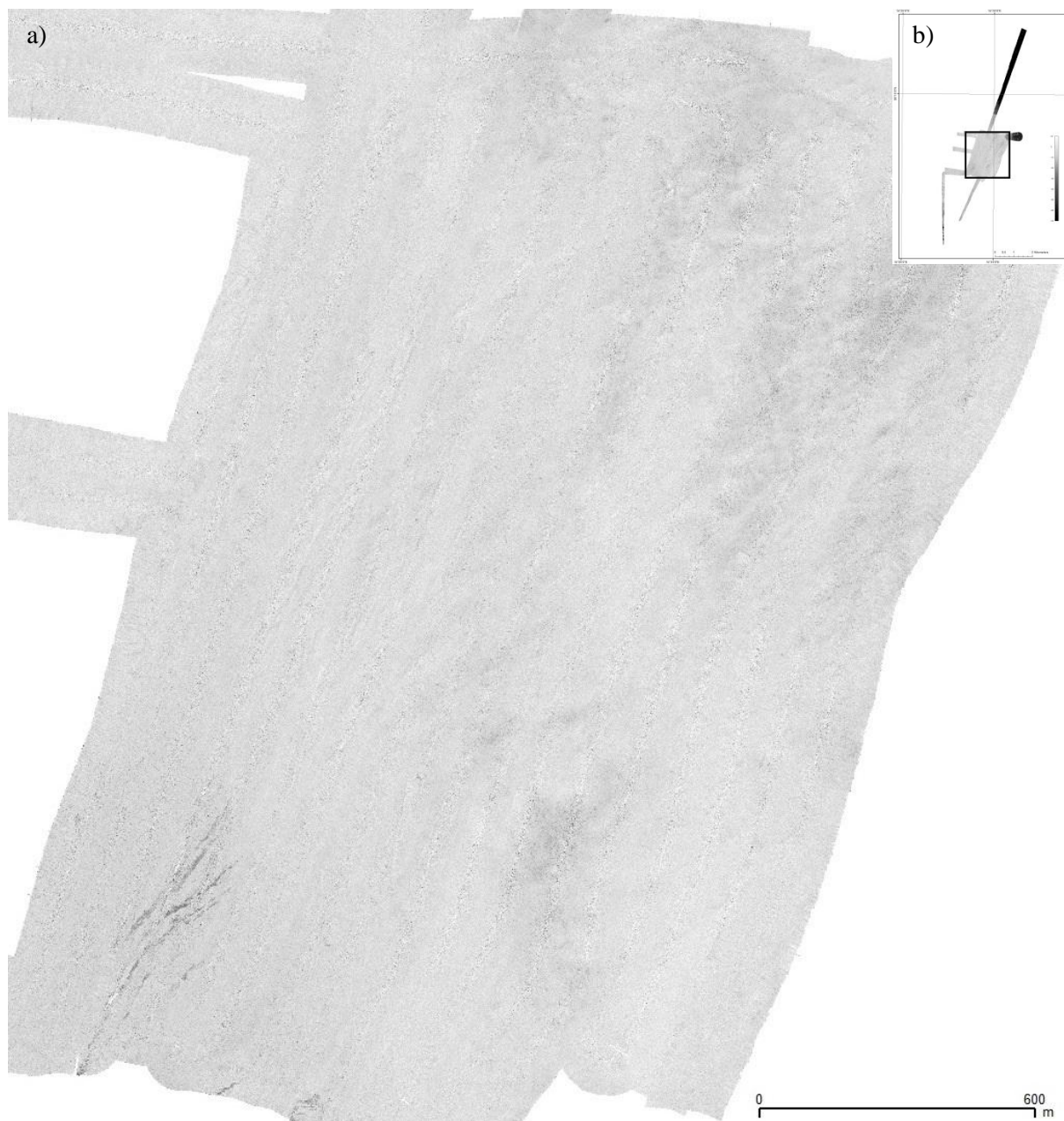
Figure 11 - Backscatter mosaic, displaying the backscatter response a) The part of the survey area that is of interest b) The entire survey area, processed and visualized using the Fledermaus software (See Appendix, Fig. B for a full-sized version). The inset rectangle shows the area in panel a).
