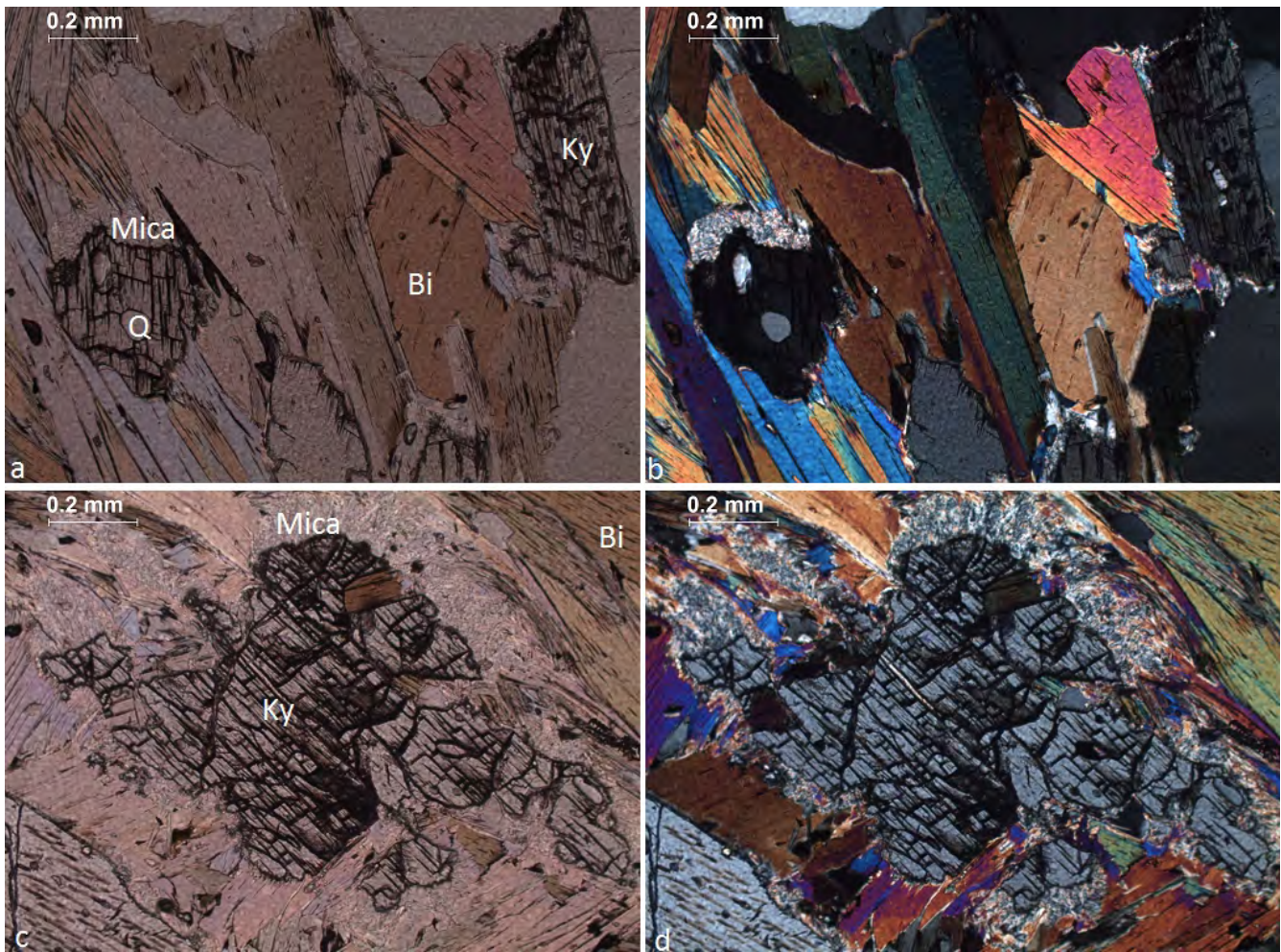
Fig. 26 The kyanite in photograph a-b has been 29% retrograded while c-d has been 46% retrograded.
