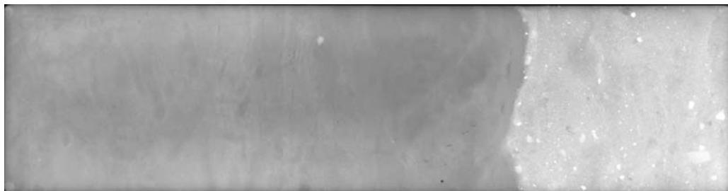
Fig. 7. X-ray photograph of grey layer lower boundary in core AO96 14-1GC. There is a distinct increase in IRD (white specks) and general grain size. Right is upward in the core. The boundary is at 166.5 cm core depth.
