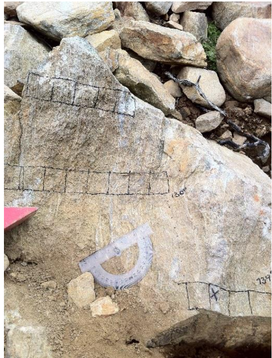
Figure 6. Picture shows profiles with 3 \times 3 \text{ cm}^2 squares on outcrop in the field.
