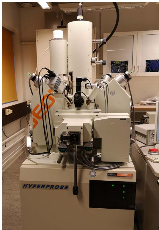
Fig. 9. Electron microprobe at Uppsala Geocentrum the 27 april 2026.
