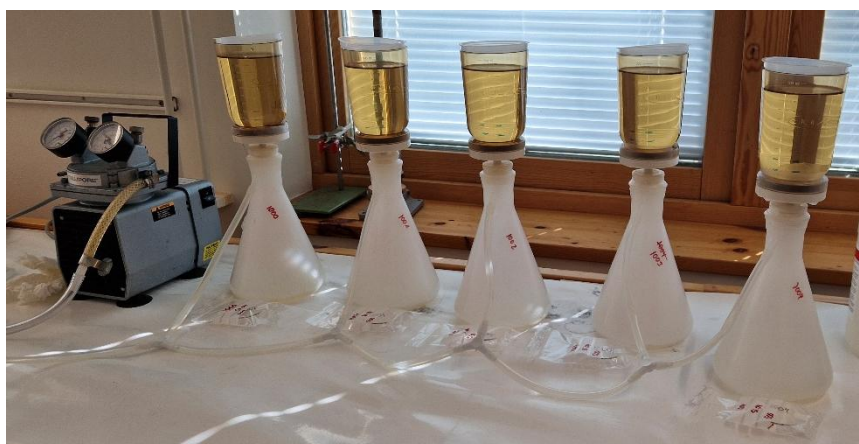
Figure 1. 0.2 \mu\text{m} filtration complete setup with PC filters, water samples, vacuum pump, beakers with filter holders, and collection flasks with water guards.
