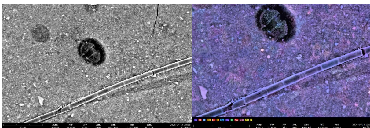
Figure 11. One example of an SEM photo from 0.2µm PC filter showing organic material with high concentrations of Si, O, C, and some trace elements.
