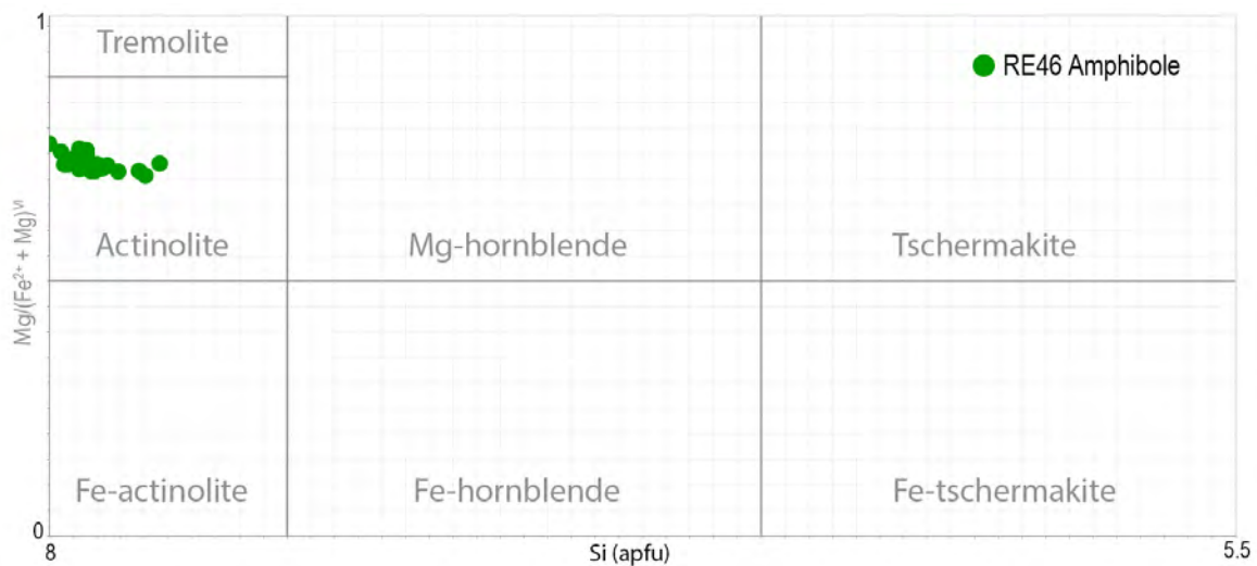
Figure 23: All amphiboles measured in this sample show homogeneous chemical composition, plotting very close together. The largest chemical difference is 0.17 Si a.p.f.u.
