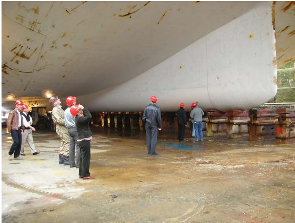
Photo 4. The acoustic transmitters and receivers of the multibeam and sub-bottom profiling system is placed in Oden's large "ice knife", which is seen in this photo. This feature diverts the broken ice to each side of the ice-breaker hull. This means that underneath the ice knife there should be less crushed ice passing than on each side of it.
