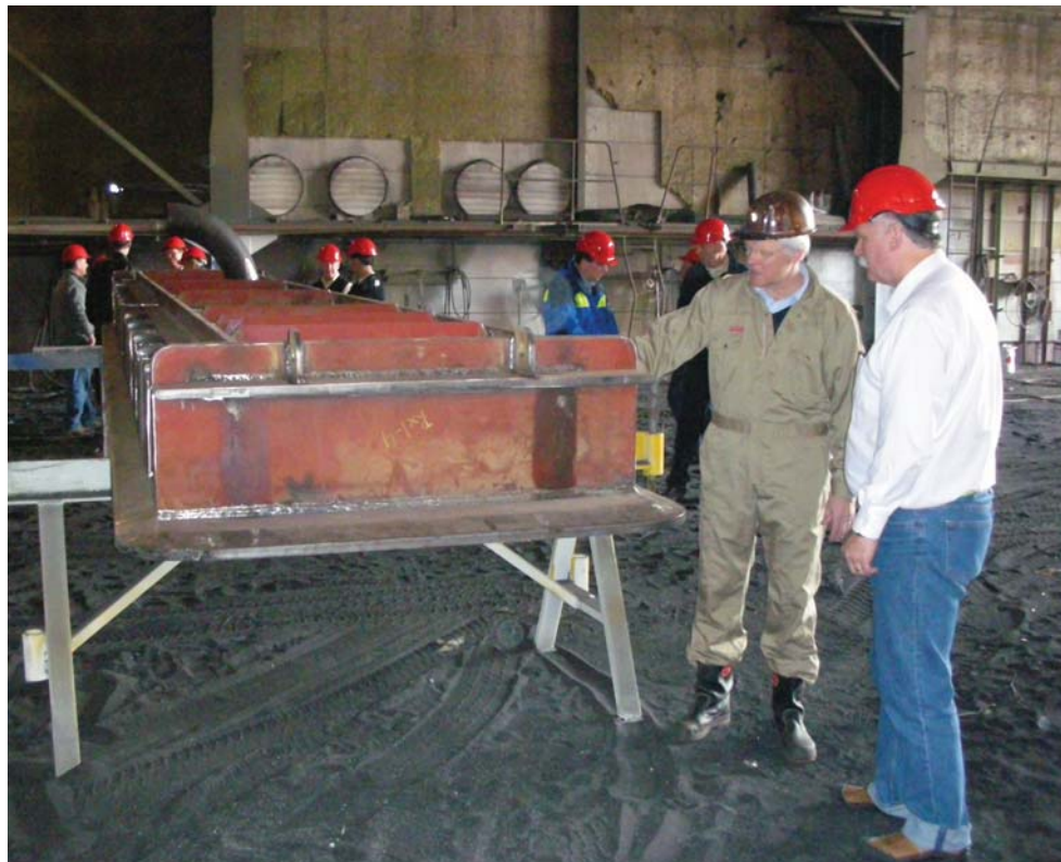
Photo 2. The constructed steel frame for the combined receiver transducer array (RX-unit) for both EM120 and SBP120. This frame was mounted in the hull of icebreaker Oden together with one frame for the EM120 transmitter and one for the SBP120 transmitter (TX-units).
