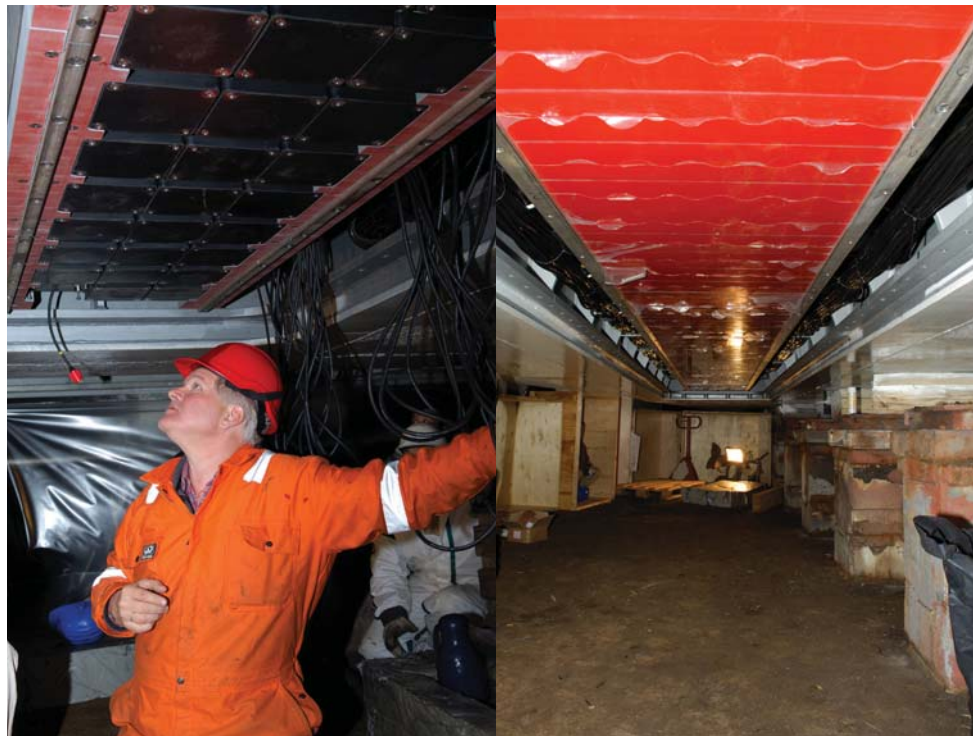
Photos 5 and 6. (Left) A portion of the SBP120 transmitting array (SBP TX-unit). This 8 m long and 1 meter wide array is mounted along ship. (Right) The 8 m long and 1 m wide EM120 transmitting array, which is mounted next to the SBP transmitting array.
