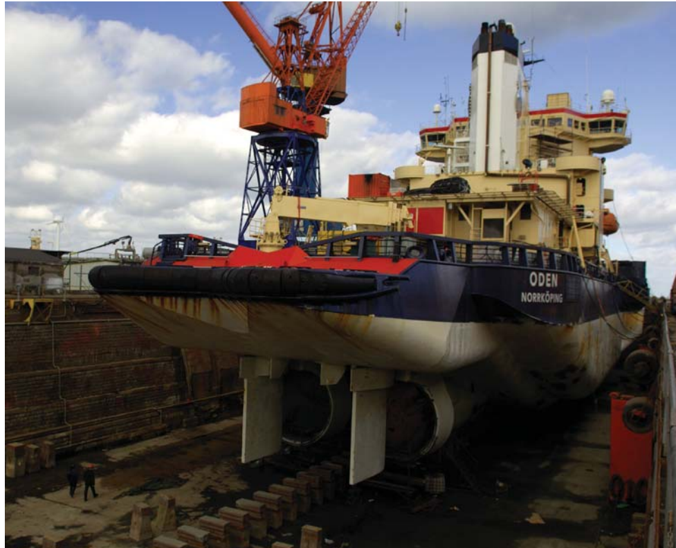
Photo 1. Icebreaker Oden placed in dry-dock at Öresundsvarvet in Landskrona. The photo shows the stern of the icebreaker and its two large (4x8 m) rudders.
