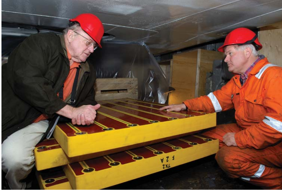
Photo 8. Both the multi-beam and subbottom profiler TX-units are covered by ice protection windows made of polyurethane plastic reinforced by imbedded titanium rods. The polyurethane later proved to have been hardened in insufficient conditions resulting in delaminating between the plastic and the titanium. These windows will be replaced by Kongsberg during the spring of 2008. The receiving array is protected by a pure titanium plate.
