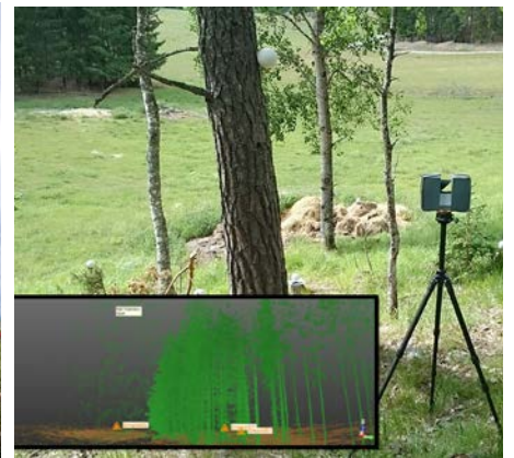
Terrestrial laser scanner set up and resulting scan (inset) to analyse forest border quality for bats in Sweden. Photo: H. Wood.
