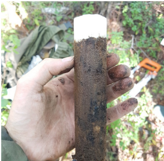
Permafrost sample with ice lens. Photo: J. Palmtag.
