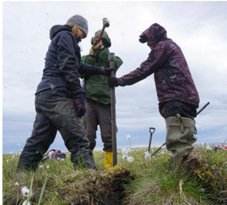
Julia Wagner is part of a team coring permafrost using a steel pipe and sledgehammer along the Yukon coast in Arctic Canada. Photo: G. Hugelius.
