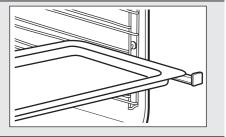
Wire shelf and deep pan together: Place the wire shelf and the deep pan together on the telescopic runner.
