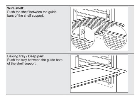
Wire shelf, Baking tray / Deep pan: Push the tray between the guide bars of the shelf support and the wire shelf on the guide bars above.
