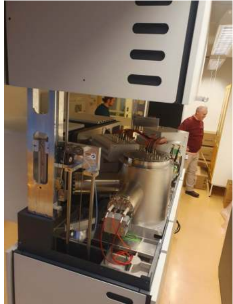
Fig. 1: The new mass spectrometer which can measure clumped isotopes.
