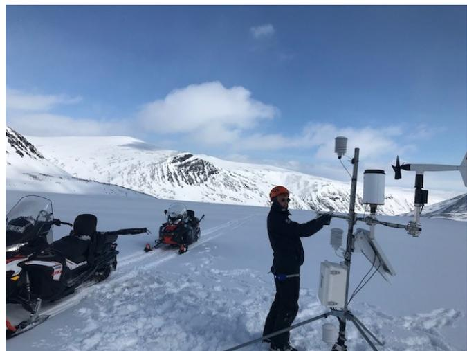
The automatic weather station is being re-mounted by research engineer Barnett at Storglaciären after the winter break.
