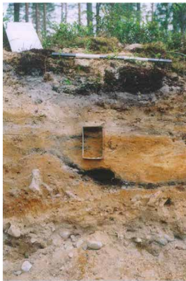
Figure 3. A Kubiena box is pressed into the profile to collect the sample Mi-3, about 3 m apart from profile 7.
