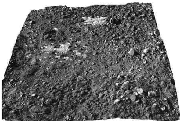
Figure 8. Scanned model of the terrace area at Skallmyran, with excavated areas. A photograph is draped on the surface. The view is from the north and covers a scanned area of approximately 65 × 50 metres.
