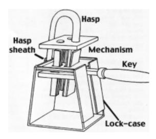
Figure 3. The parts of a Type II padlock.
