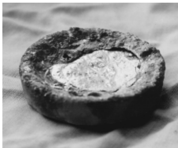
Figure 3. One of four experimental trays made by the author. The silver/lead alloy has solidified in the tray, showing its position in the central depression eroded by the lead. Width 63 mm. Photo: Anders Söderberg.
