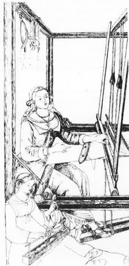
Fig.1. Illustration of the front and interior of a treadle loom showing hanging pulleys and under them, two shafts which regulate the warp-threads and the treadles. After a painting by Pinturicchio (d. 1513). After Grenander Nyberg.
