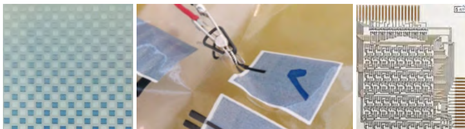
Figure 1. Left: Screen printed passive matrix addressed electrochromic display with 17 grayscale levels. 1 Middle: all-organic electrochromic displays screen printed on transparent nanocellulose-based substrates. 2 Screen printed OECT-based shift register. 3
