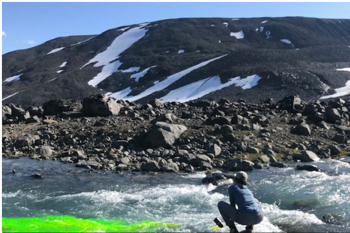
Discharge measurements at Lillsjön outlet. Photo by Granebeck.
