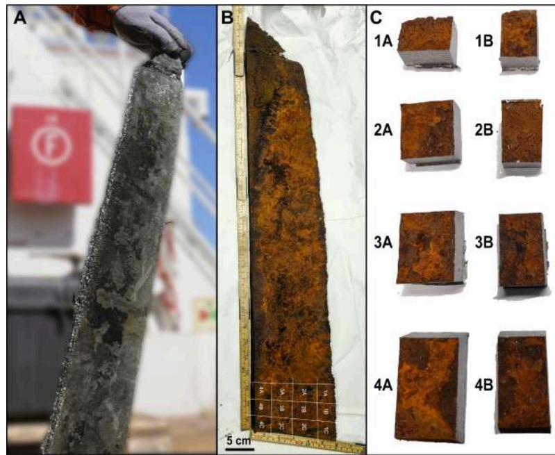
Figure 6. Subsampling of the cut-out steel plate. (A) Metal surface covered by black precipitates before and just as it was brought up to the fully oxygenated surface environment. (B) Metal surface after exposure to air. (C) Subsamples used for SEM-EDS analyses (1A-4A) and subsamples used for element analyses (1B-3B).
