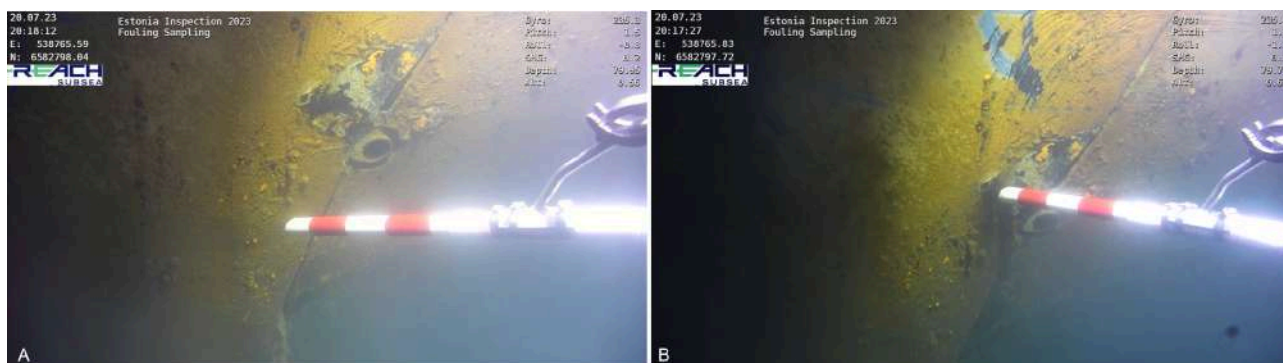
Figure 4. Photos showing the suction sampler (Bluefield Geoservices) attached to remotely operated underwater vehicle (ROV).
