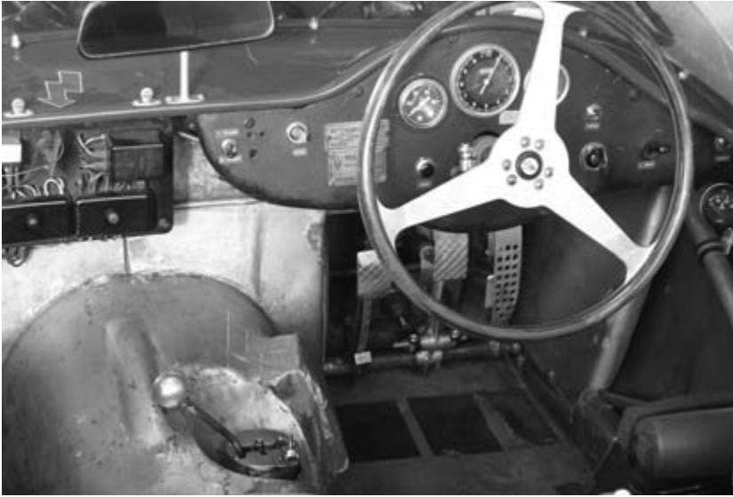
Figure 43. The steering wheel, pedals, gear lever, fuses, and switches: everything speaks of racing in this Maserati 300S interior.
