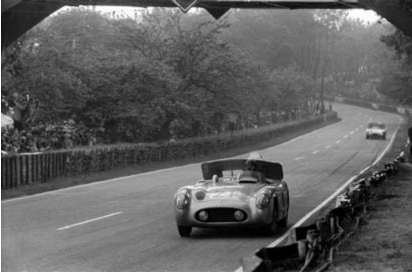
Figure 39. Kling and Simon's Mercedes with its airbrake opened at the ill-fated 1955 Le Mans race (copyright Getty Images).
